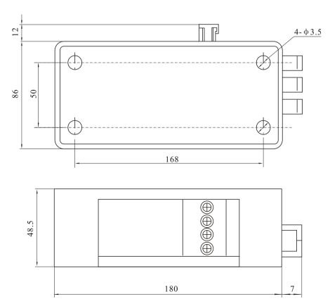
Figure 10D (power module overall and mounting dimensions figure)
