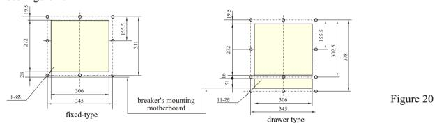
●ZW1-3200~6300 (except 4000/4 ) door frame inner dimensions and mounting hole, hole size see figure 21
