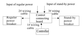
Figure 24: Wiring schematic map for users
