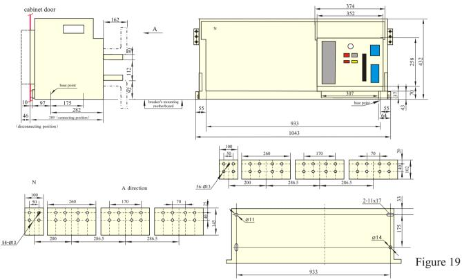
ZW1-2000、ZW1-4000/4 door frame inner dimensions and mounting hole, hole size see figure 20
