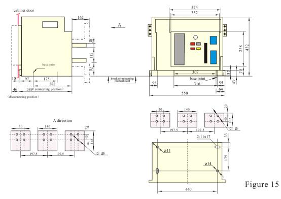
•ZW1-4000/4-type overall and mounting dimensions (see figure 16)(drawer type)
